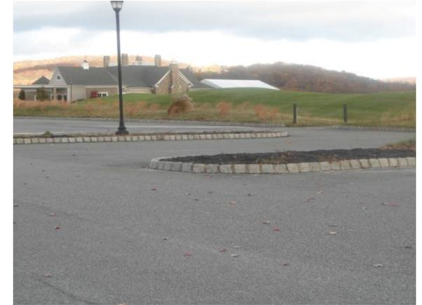
Parking islands can be replaced with tree filter boxes to capture, treat, and infiltrate stormwater runoff and improve the aesthetic of the parking lot. A preliminary soil assessment suggests that the soils have suitable drainage characteristics for green infrastructure.
