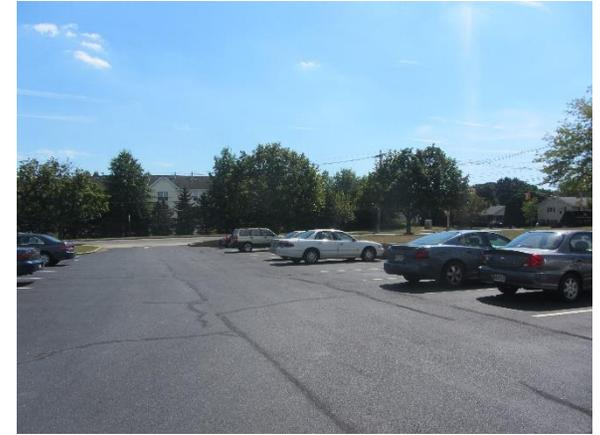
Parking spots to the west of the building can be replaced with porous asphalt to capture and infiltrate stormwater. Rain gardens adjacent to the building can capture, treat, and infiltrate roof runoff. A preliminary soil assessment suggests that the soils have suitable drainage characteristics for green infrastructure.
