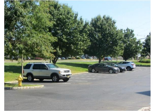
Parking spots in front of the building can be replaced with porous asphalt to capture and infiltrate stormwater runoff. Downspouts from the roof can be disconnected and directed into a rain garden. A preliminary soil assessment suggests that the soils have suitable drainage characteristics for green infrastructure.
